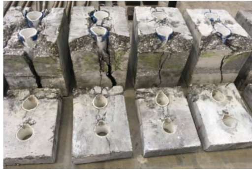
Figure 1.9 Failure mode of friction failure mode
